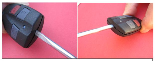
Use small flat screw-driver to open remote key on the split line separate it into two parts and remove worn key pad.
